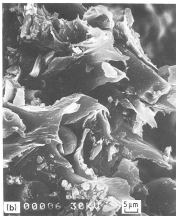
Figure 12 Comparison of fracture surfaces obtained on material 1 in (a) the tension part and (b) in the compression part of the samples. The flexion test was performed after 39 days of ageing at 70°C and 100% r.h.
